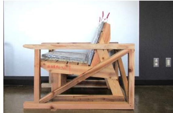
Photo3 Chair and armrest measuring instrument
