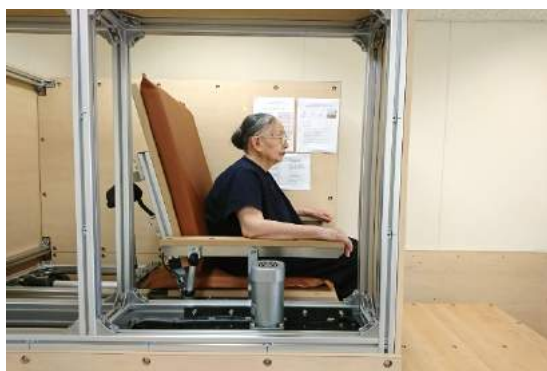
Photo2 Chair measuring device
